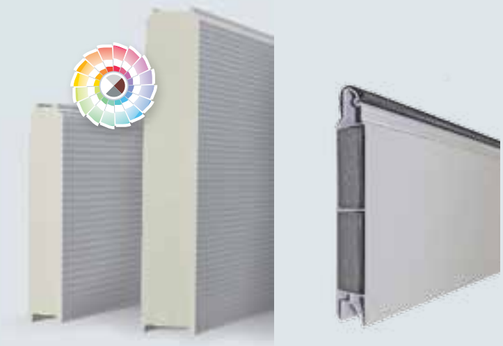
Double-skinned steel sandwich slats with thermal break in two thicknesses: 42 mm (1-5/8"), 67 mm (2-5/8"), and acoustic slat
