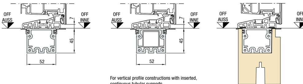
For vertical profile constructions with inserted, continuous tubular supports
