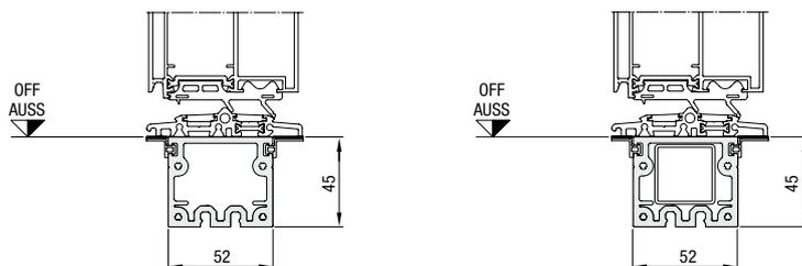
For vertical profile constructions with inserted, continuous tubular supports
