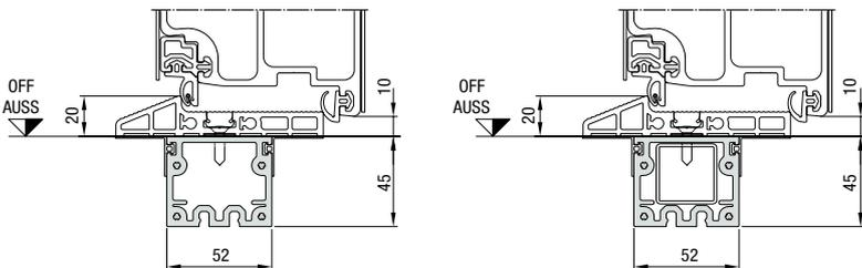
For vertical profile constructions with inserted, continuous tubular supports
