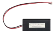
Battery unit For control 545 / 560 incl. batteries; to buffer the time and date of the control if the mains voltage supply is interrupted for longer than the standard buffer of 60 hours
