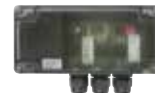
2-channel relay receiver HET-E2 24 BS 2 volt-free relay outputs for choosing the direction, one 2-pin input for volt-free Open and Close limit switch reporting (for querying the door position)
