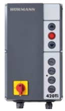
Combination control 420 Si / 420 Ti Combination of the door operation with the operator WA 300 R S4 / WA 300 AR S4 and a standard dock leveller control; Advantages: • Easy to fit • Inexpensive • Compact • Suitable for hinged lip (420 Si) and telescopic lip dock leveller (420 Ti) • Optional: Integration of the OPEN limit switch reporting for dock leveller release
