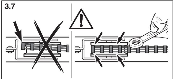
4. The toothed belt must be located on the centre of the return pulley. If required, push to the centre.
