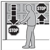
1. Stop the door with both hands while it is **closing**. The door system must stop and initiate the safety reversal.
