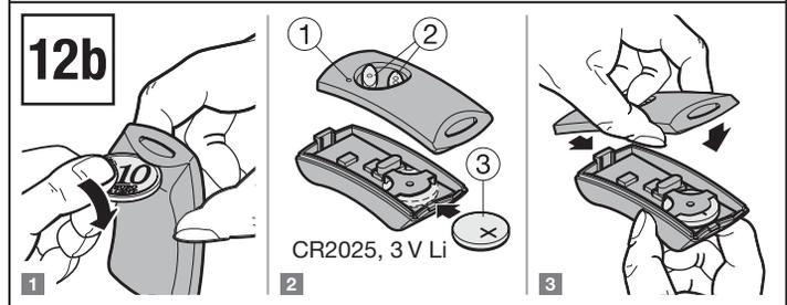
**4.2 Inserting/changing the batteries**
