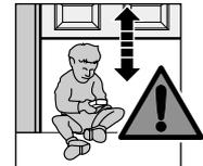
Wait until the door has come to a complete halt before entering the door's range of travel. Before driving in or out of the garage, make sure that the door has opened fully.
