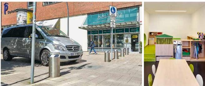
Authorised road users can let the bollard sink into the ground using a hand transmitter.
