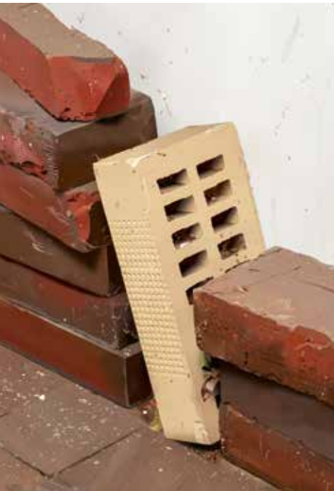
Extruded brick and water-struck brick, thin format, grouped, courtyard
